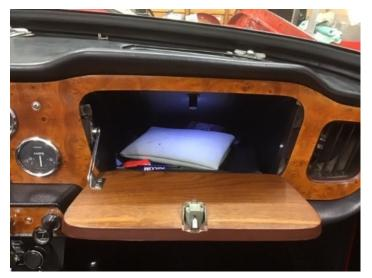
The glovebox had to be removed to replace crumbling heater box hoses under the dash, which reminded me that I can never find anything in the glovebox. This would be the perfect time to install a light! I found an LED unit that lights up the entire box and takes up so little current that I wired it to have power whenever the lights are on. An easy fix.
