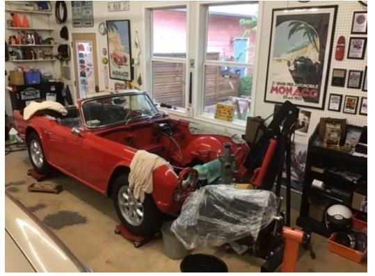
The engine and transmission came out in late-March. They, and everything near them in the car, was covered in 20 years of road grime and oil/ grease binder. Cleaning and disassembly revealed more things that needed attention. The front seal housing on the
